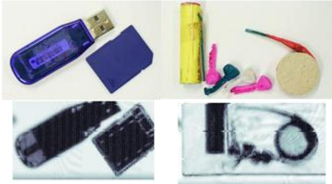
Fig. 2 Visual images (top) and THz images (below) of objects screened at 0.82 THz. The images were captured with an integrated Silicon solution; no expensive THz equipment was required.
